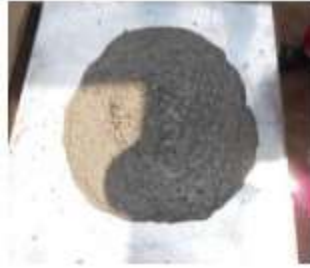
Slump flow test
